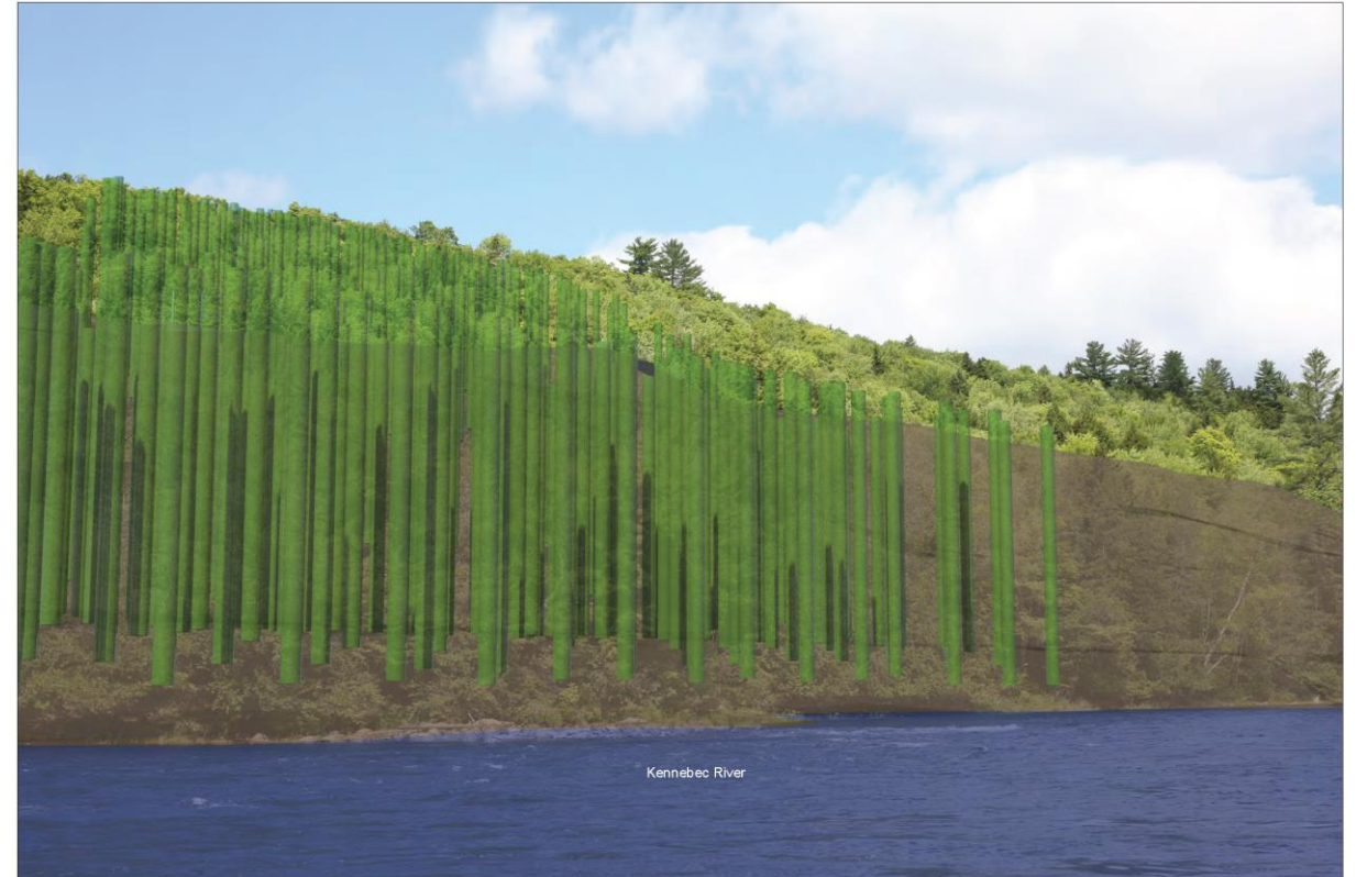
COMPUTER MODEL A-3: This image shows the computer model (terrain and 75' tree cylinders) overlaid and registered with the Existing Conditions photo. The preserved vegetation on the hillside will completely screen the West Forks Termination Station from the Kennebec River.
